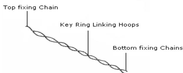
Before you start please note, if you are attaching a Chain to a 54" Mace then you will need to remove the top two loops including the two key ring linking hoops from the Chain, but remember to reattach the top fixing length of Chain to the top of the Chain assembly.
